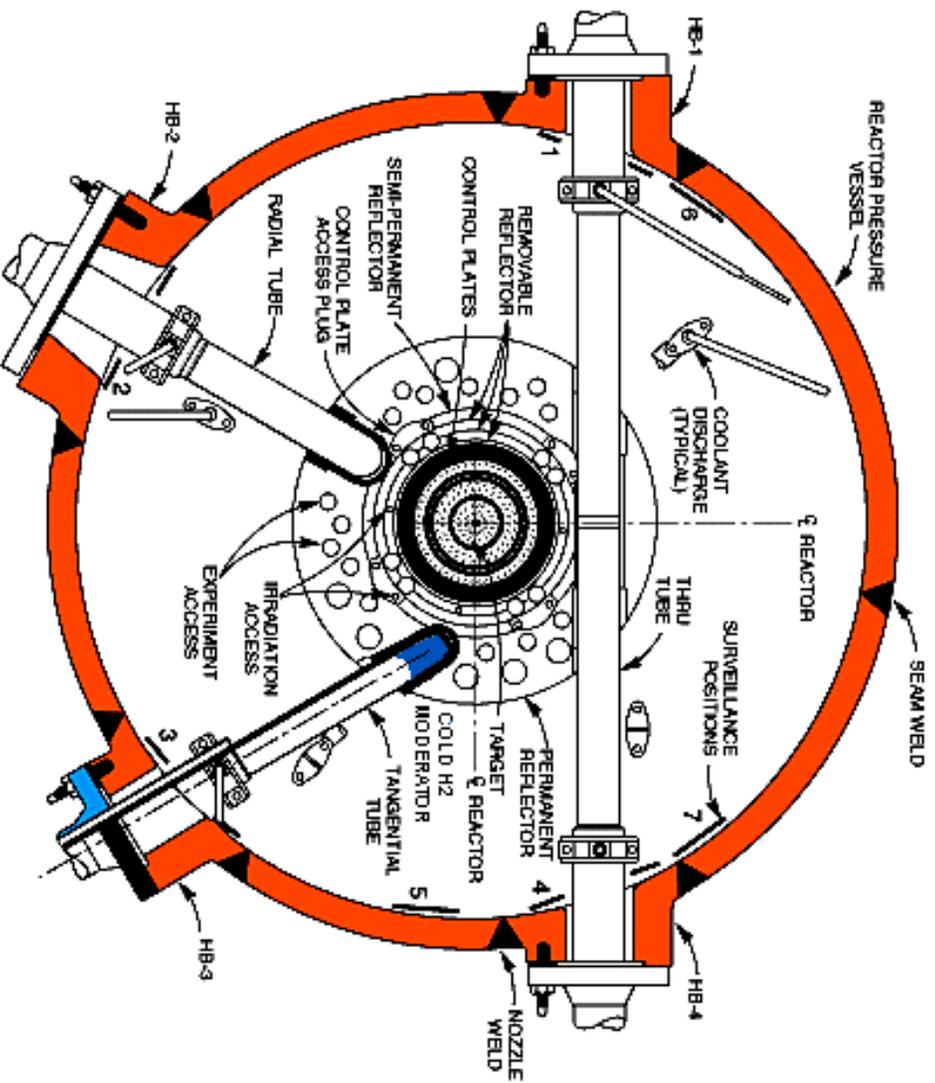
Section view of ORNL/HFIR reactor. For  $n \rightarrow \bar{n}$  search experiment the cold supercritical hydrogen moderator should be installed in the HB-3 beam tube.
