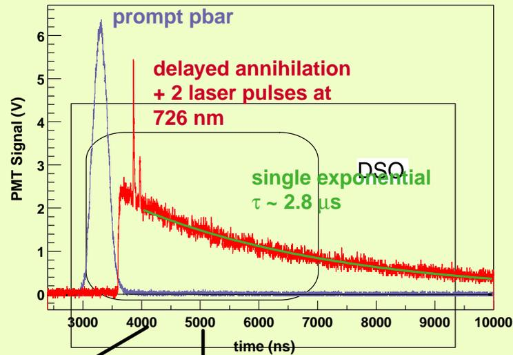
Analog Measurement of Delayed Annihilation using Cerenkov counters and digital oscilloscope
