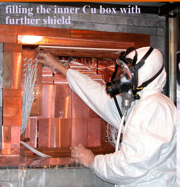
closing the Cu box housing the detectors
