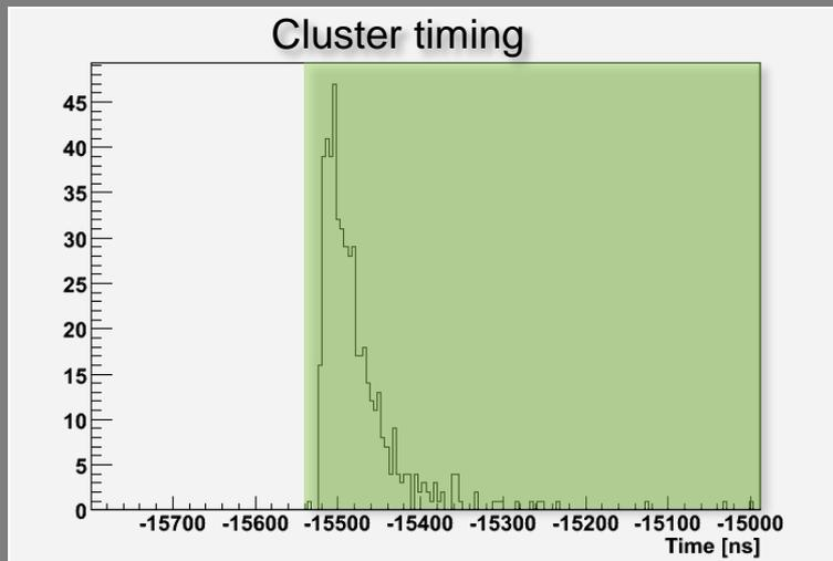
PMT time-of-flight distribution used for **position** reconstruction
