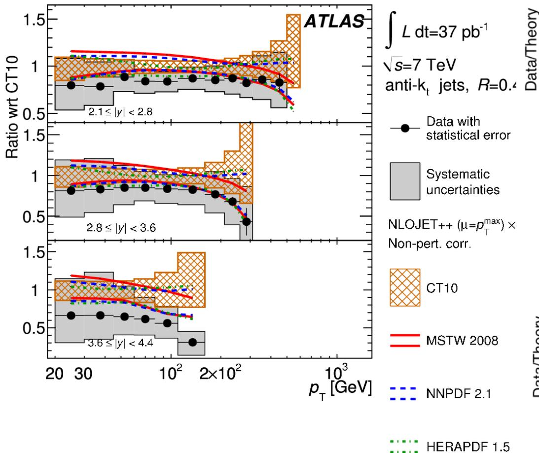
**Data at the edge of the phase space in the forward promise to further constrain the gluon PDFs (in a region with limited  $p_T$  where no new physics is expected)**
