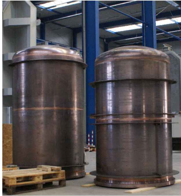
Cryostat shields @ factory
