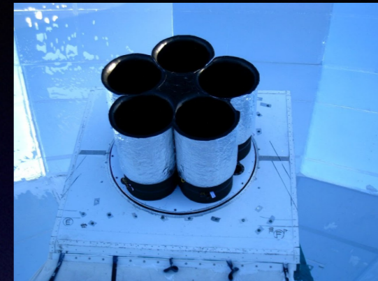
Keck Array: Phased antenna array, TESSs, 150 GHz
