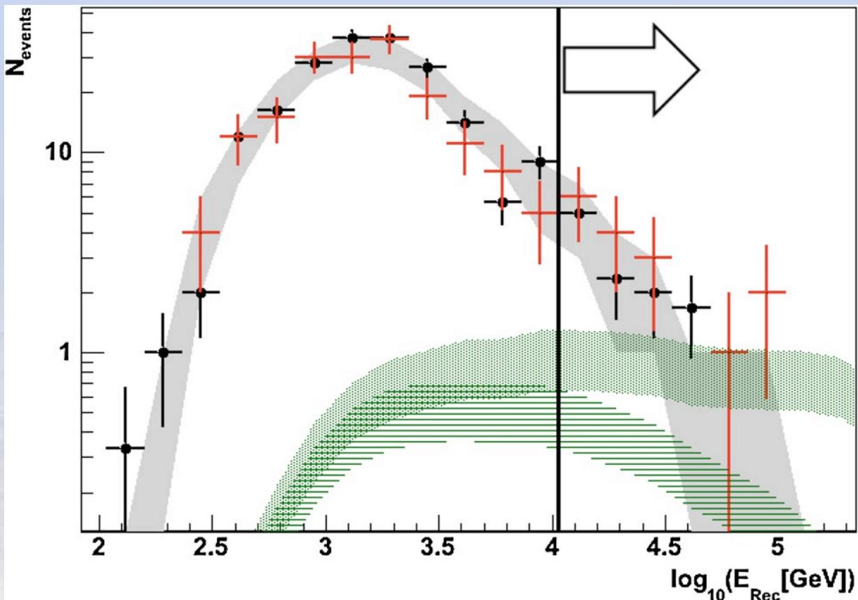
Distribution of the reconstructed energy of the events after the final cut on : events in on-zone (red crosses), average over off-zones (black circles), 68 % confidence area given by the total background simulation (grey area), expected signal from the Fermi bubbles without neutrino-energy cutoff (green dotted area) and 50 TeV cutoff (green cut is represented by the black line with a dashed area). The chosen  $E_{\text{Rec}}$  is represented by the line with the arrow
