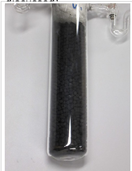
carbonaceous filter material
